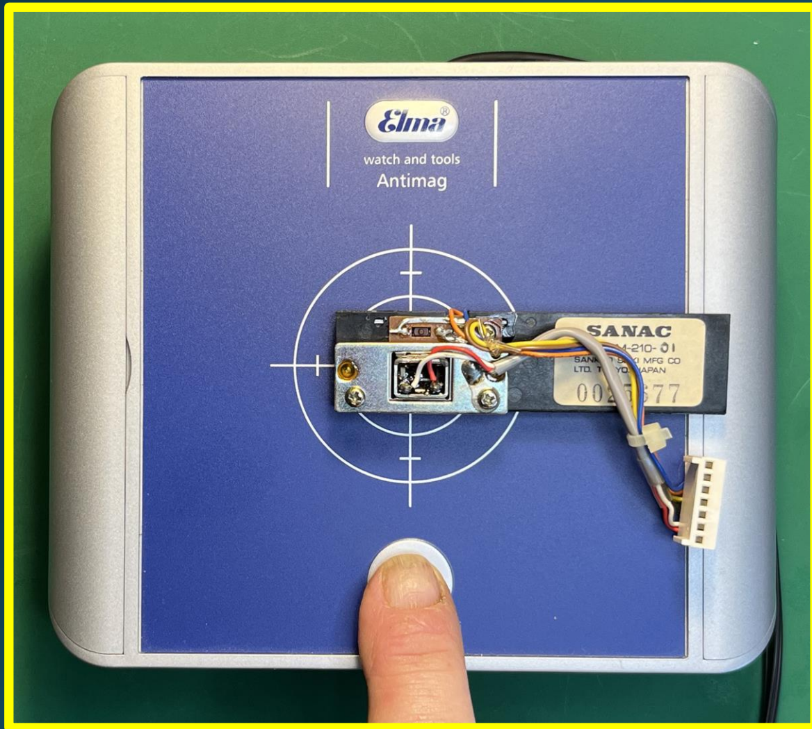
Demagnetizing the play / record head.
